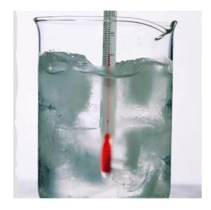
Circle students melted ice over a low bunsen flame and observed that as the ice melted from a solid to a liquid state there was no temperature change. Then when water turned from a liquid to a gas state there was once again no temperature change. This is because energy was being used to break bonds as it turned from one state to another!
